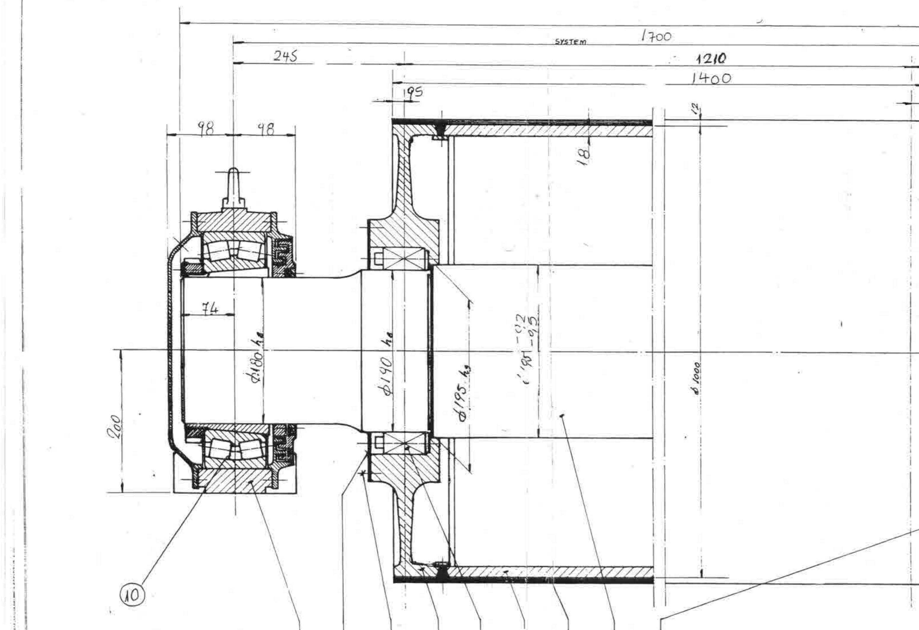
Technical drawing of a mechanical part, likely a bearing housing, showing various dimensions, material thicknesses, and assembly details.
