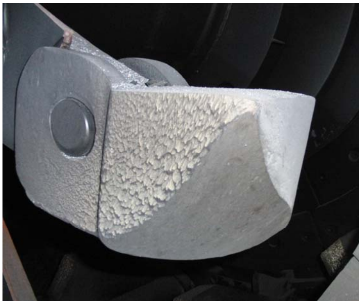
Picture of a worn beater head
