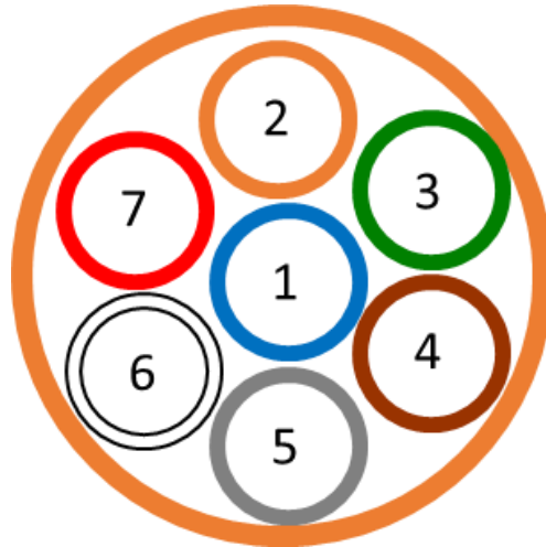
Figure 6 - Example of 7x10/14 DB Microducts Bundle
