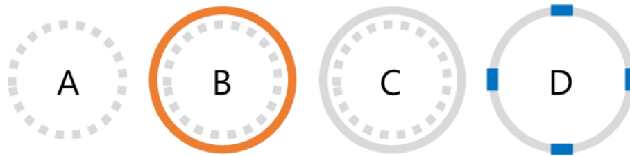
Figure 3 - Example of DB (Single Layer Microduct transparent, A, Double Layer Microduct orange, B, and UV resistant Double Layer Microduct grey, C) and DI (D) Microducts
