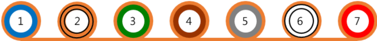
Figure 4 - Example of 7x10/14 DB Microducts Linear Bundle
