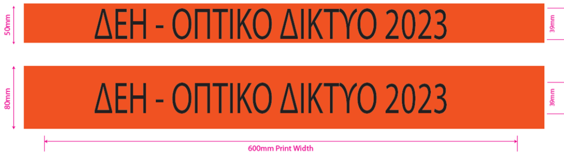
Figure 28 - Print dimensions and positioning for 5 cm and 8 cm marking tape
