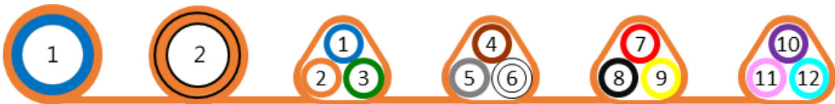
Figure 5 - Example of 2x10/14+4x(3x4/7) DB Microducts Linear Bundle
