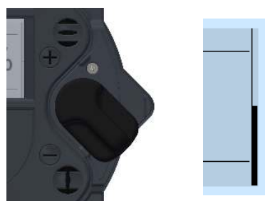
Figure 51: Full switch flip (it will jump to the end of the menu)
