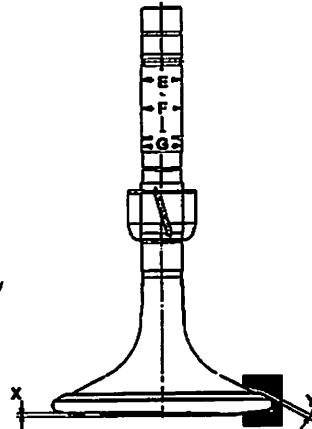
Wear Y : [mm] Maximal allowable grinding Y: 3,00 [mm]
