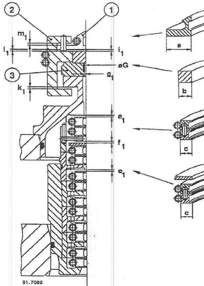
When checking the clearance at  $i_1$  the scraper ring (1) must lie on guide ring (3)
