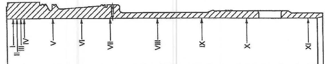
**Before measuring, the measuring point "I" should be adjusted to be approximately in the middle of the uppermost ring at TDC**
