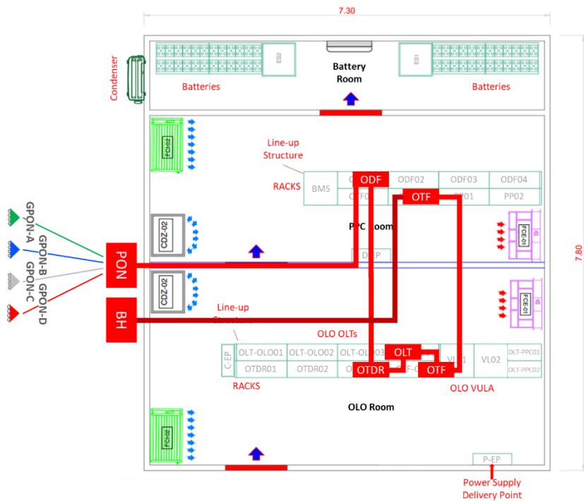
**Figure 3 - Logical path connecting equipment in indoor POP for Passive Services**
