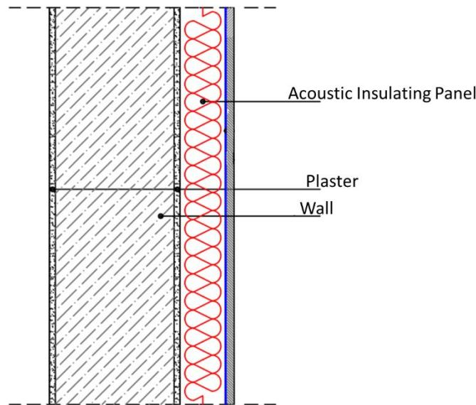
**Figure 4 - Example of acoustic soundproofing**
