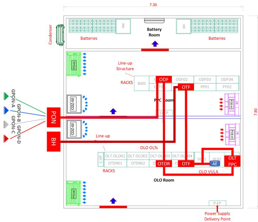
**Figure 2 - Logical path connecting equipment in indoor POP for Active Services**
