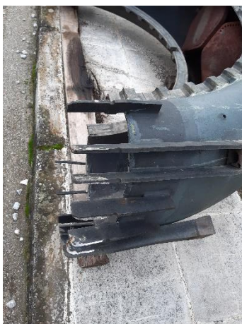
Split Line Ribs – Typical disassembly damages
