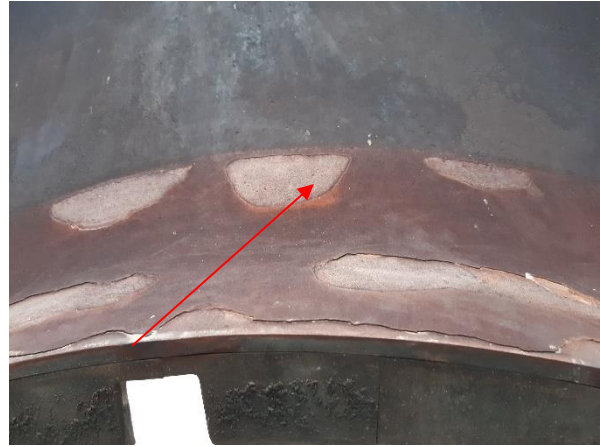
Missing TBC (post operation)
