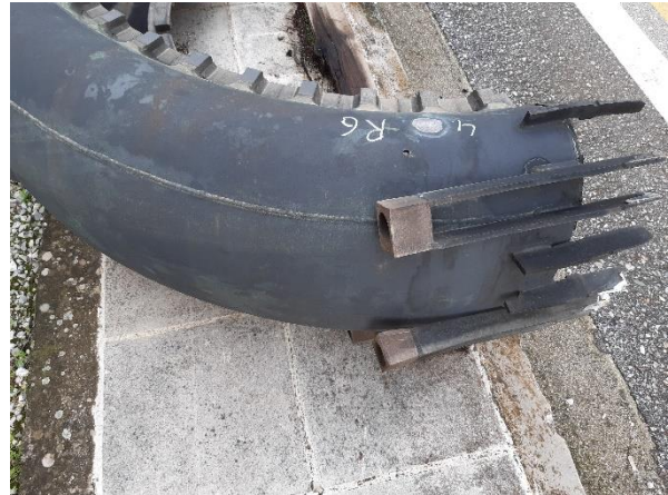
Split line – Fixation (typical disassembly damages)
