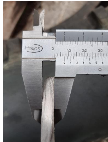
Body Wall Thickness – material sample 7,3 - 7,5mm
