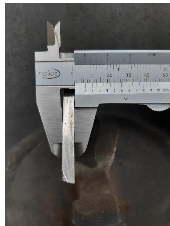
Body Wall Thickness – material sample 6,8 - 7,0mm
