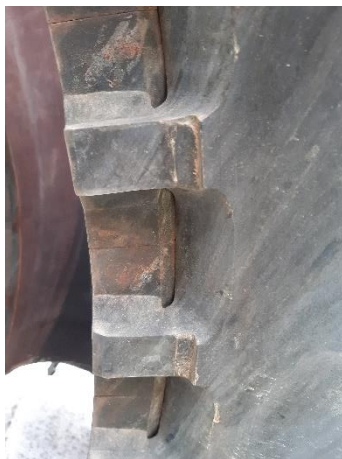
Turbine Suspension Ring – fretting contact surface (1-2mm)
