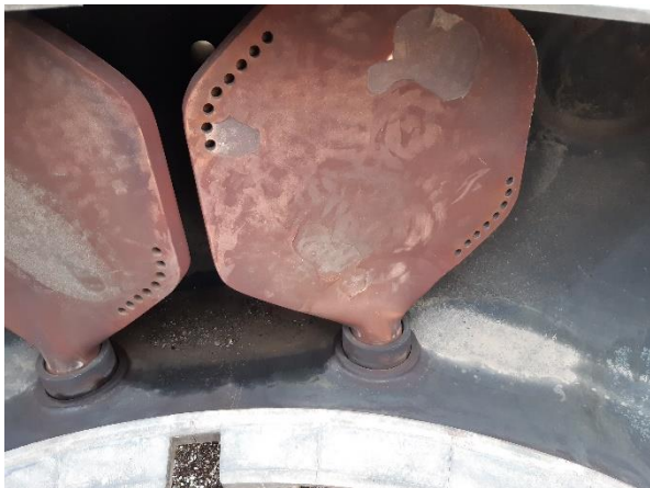
Turbine Suspension Ring – fretting contact surface (2-3mm)
