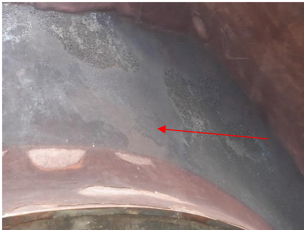
Split Line Overview – typical disassembly damages
