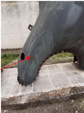
Huge Deformation main body Compressor Side
