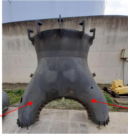
Huge Deformation main body Compressor Side
