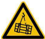
Danger of falling objects
