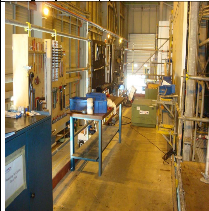
Placing of workbench and Shadow Board
