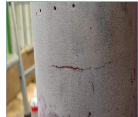
Crack at mixed weld seam
