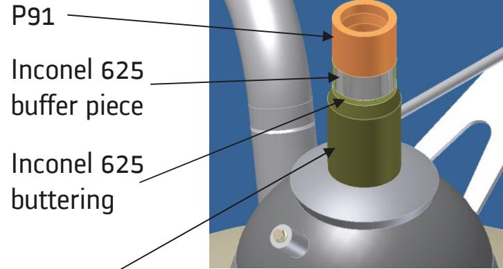
**Alstom delivery allows LBG92 steam line connection with SS316 or P91**
